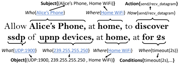
Fig. 8: Rule to allow discovery of the WeMo plug. The WeMo has 2s to reply to the phone’s broadcast discovery messages.
